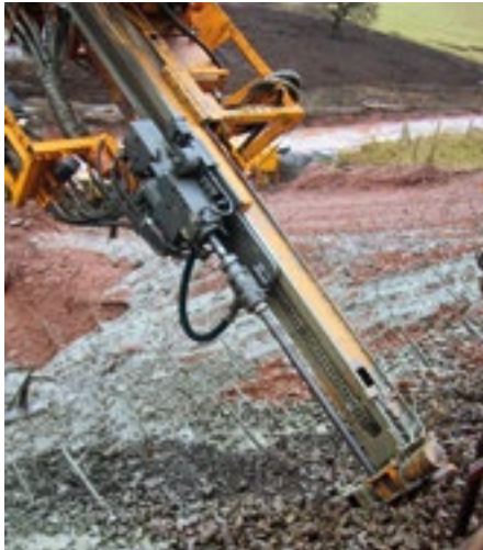
Rotary percussive top hammer (hydraulic)
