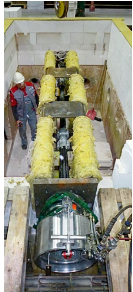
PTI Load capacity test at 300°C
